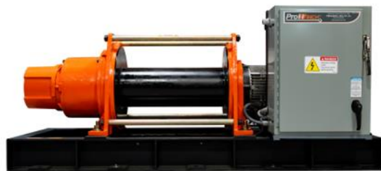
8000 lb Heavy Duty Winch 240V 3 y 480 V Phase SEW UL Motor UL508A Control Variable Speed Made in USA
